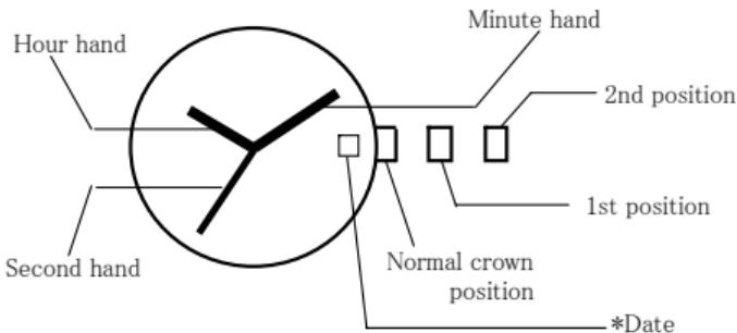
Some watches have a screw-in-crown: if it doesn't come out , rotate the crown clockwise until the release. At the end of the adjustments close the crown. Do not use the watch when the crown is open.
