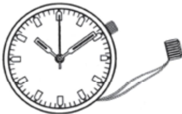
Unscrew the crown cover before adjusting the time
