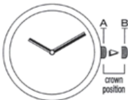
**1** Unwind the crown (if with screw mechanism) • **2** Pull out the crown to position B • **3** Wind the crown in any direction to adjust the time • **4** Push the crown back to position A • **5** Rewind the crown (if with screw mechanism)
